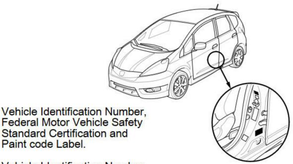
Vehicle Identification Number, Canadian Motor Vehicle Safety Standard Certification and paint Code Label.
